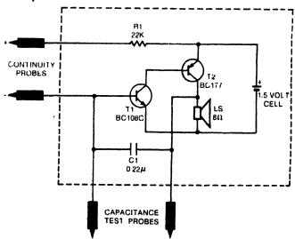
The versatile continuity tester circuit which has numerous applications.
